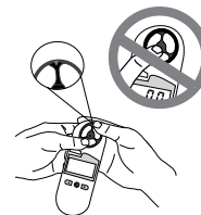
Replacing the Impeller
