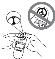
Replacing the Impeller
