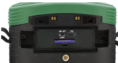
Grasp spring loaded buttons on SD card door edges and pull
