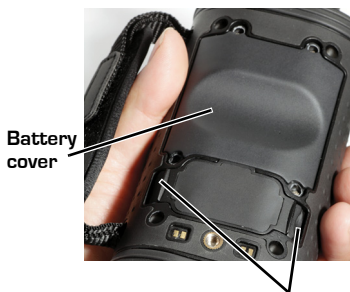
Grasp SD card door edges and pull
