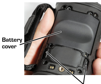
Grasp SD card door edges and pull
